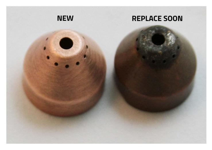
The shield cap orifice should be round and smooth. Because it is close to the work piece, it can suffer from spatter, and nicks. You can clean it with a non-metallic kitchen abrasive pad (don't use sandpaper), if it is not badly burned, dented, or cracked around the orifice. When you remove the shield cap, check the O-ring (if present) and its lubrication.
