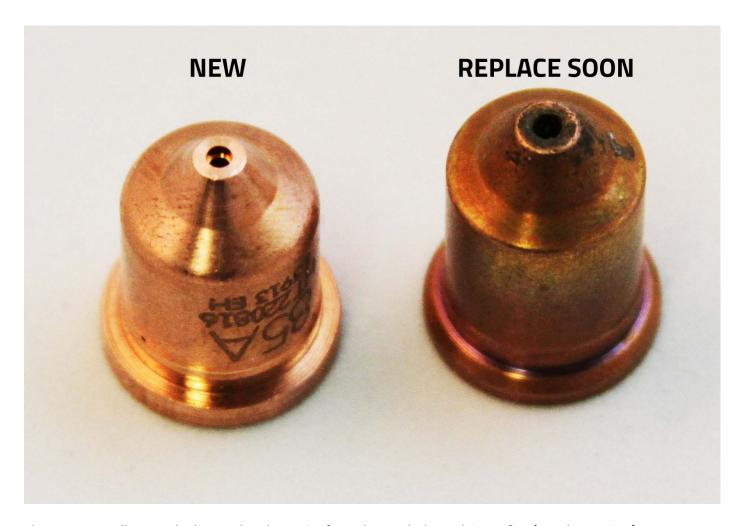
The copper or alloy nozzle directs the plasma jet from the torch through its orifice (nozzle opening). Larger amperage nozzles will have larger orifices, but any new nozzle will have an orifice that is not only round, but has sharp, not rounded, edges. Check the orifice and replace it if it shows any oval or oblong shape.
