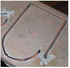
Instances where the metal was not fully cut indicate a few different problems. If the ground clamp was not properly attached to the material this can happen. A similar cut can happen if there was a drop in air pressure, moisture in the air line, or a drop in power. A third cause is if the torch contacts the material, most plasma cutters will go into a low power mode when this happens causing the cut not to penetrate all the way.
