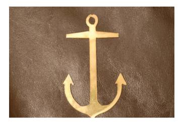
In some cases the slipping in one direction will be offset by slipping in the opposite direction of travel. This allows the part to be cut out but the tool path was not followed correctly. Set screws, belts, gear spacing, and square of the table should be checked.
