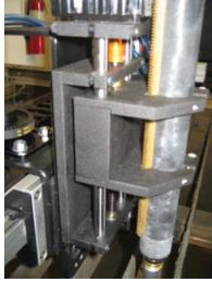
An automatic voltage height control relies on a connection to the plasma cutter to receive a raw arc voltage signal. This is used to maintain the height of the torch from the work piece. While cutting if the height climbs away from the material the "set voltage" is too high. Likewise if the torch tends to dive into the material the "set voltage" is too low.
